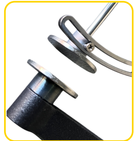
HAND LAPPED DISKS DIAMETERS 20, 30, 50MM
