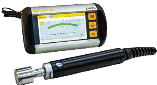
SmartPlug with transducer holder and standalone display
