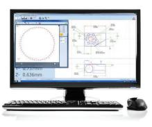
Every time a component is inspected, a programme for measuring subsequent components is automatically created. The software also calculates 'safe' moves between features, even when the probe is indexing – just another thing that the operator doesn't have to worry about!
